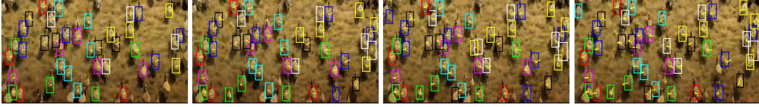
Figure 4.10: Multiple object tracking results shown on frames excerpted from the sequence of Zebra. Different colors correspond to different objects (only 8 colors are adopted so some boxes are of the same color), the yellow lines represent trajectories.
