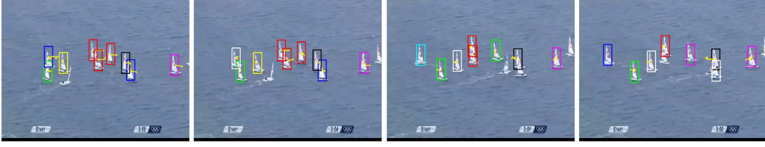
Figure 4.15: Multiple object tracking results shown on frames excerpted from the sequence of Sailing. Different colors correspond to different objects (only 8 colors are adopted so some boxes are of the same color), the yellow lines represent trajectories.
